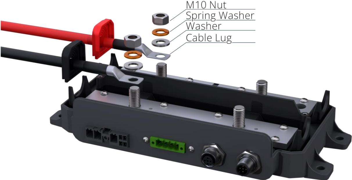
Figure 18 - Alternator power cables
